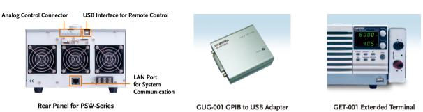
The PSW-Series provides USB Host port in the front panel for easy access of stored data, such as test script program. In the rear panel, a USB Device port is available for remote control or I & V data logging of power output through a PC controller. The LAN interface, which meets DHCP standard, is provided as a standard feature of the PSW-Series for system communications and ATE applications.
