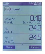
The device displays the U coefficient, the surface temperature, the ambient temperature and the external temperature.
